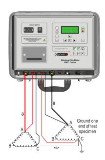
Using RMO60T's Tap Changer menu, the power transformer winding resistance of individual tap positions can be measured. Also, you can check whether the on-load tap changer switches without an interruption. The RMO60T current output injects a constant current into a power transformer. This current and voltage value is measured, and the winding resistance is calculated.
