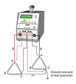
Using RMO10T's TapChanger menu, the power transformer winding resistance of individual tap positions can be measured. Also, you can check whether the on-load tap changer switches without an interruption. The RMO10T current output injects a constant current into a power transformer. This current and voltage value is measured, and the winding resistance is calculated.
