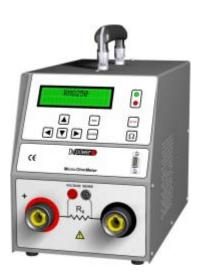
International standards, when measuring circuit breaker contacts call for currents in the order of 50A (IEC 56, now IEC62271-100) or minimum 100A (ANSI C37.09) up to the breaker's nominal current (which would be a manufacturer's preference).
